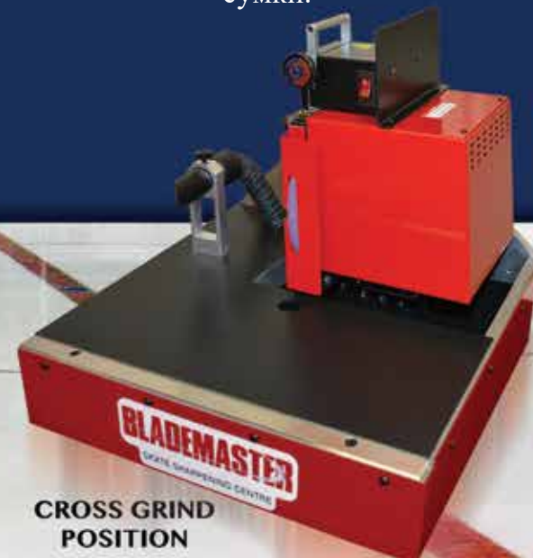
Head pivots between cross-grind and finishing positions
